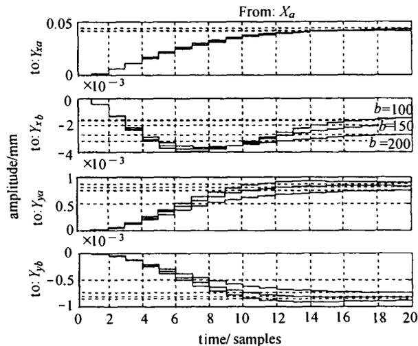
Fig. 4 Unit step respond in  $X_a$  direction when “ $b$ ” chose different value,  $a=1000$
