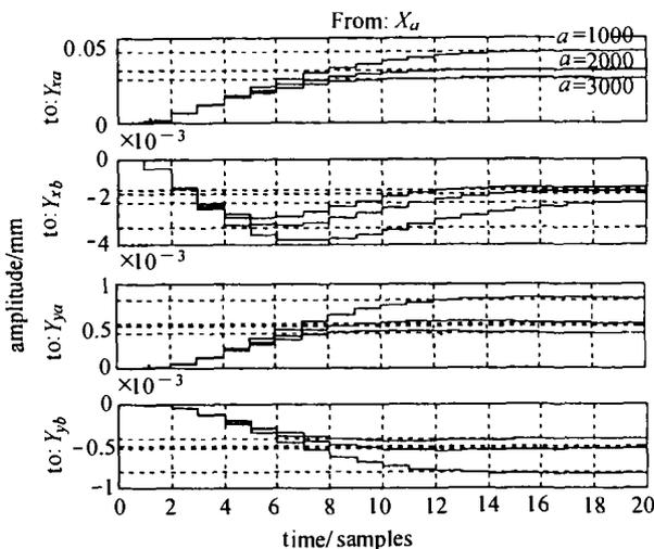
Fig. 3 Unit step respond in  $X_a$  direction when “ $a$ ” chose different value,  $b=100$
