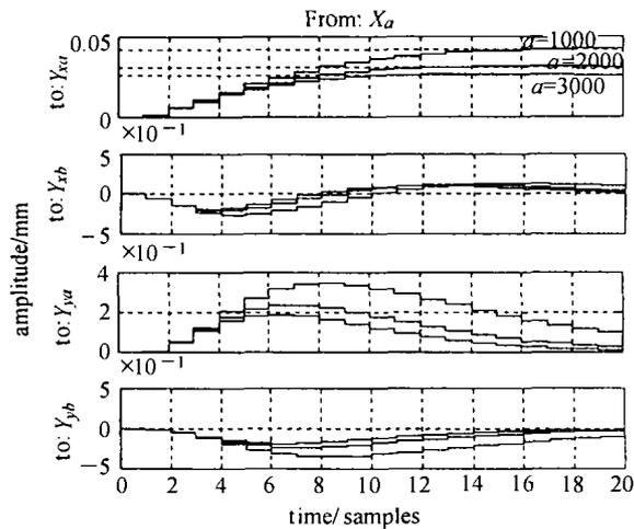
Fig. 5 Unit step respond in X<sub>a</sub> direction when "a" chose different value, b=100,coupling is ignored
