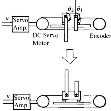
Fig. 4 Illustration of the control problem for the parallel cart-type double inverted pendulum
