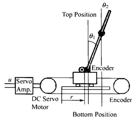
Fig. 2 Serial cart-type double inverted pendulum system
