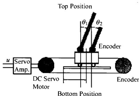
Fig. 1 Parallel cart-type double inverted pendulum system
