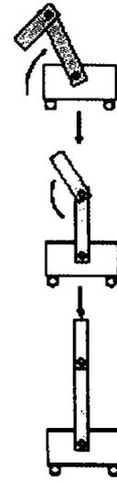
Fig. 5 Illustration of the control problem for the serial cart-type double inverted pendulum
