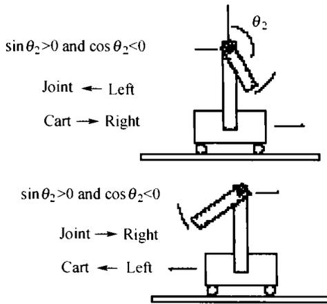
Fig. 6 Swinging up the second pendulum
