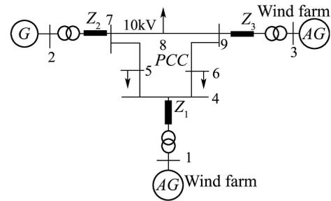
Fig. 9 Connection circuit between wind farm and weak grid
