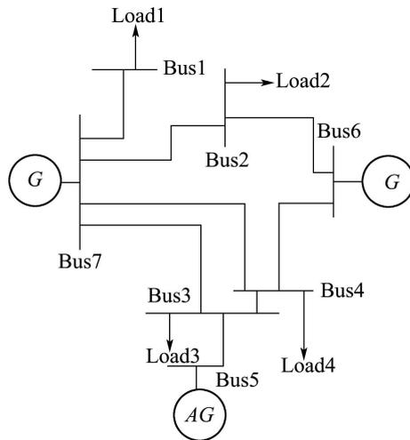
Fig. 13 Diagram of wind farm connected to “weak grid”
