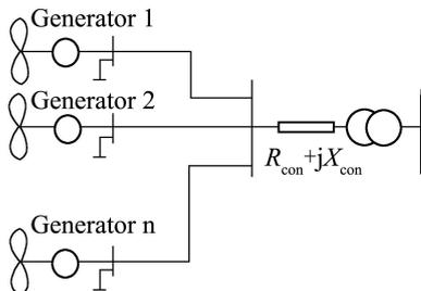
Fig. 3 Wind farm with “constant speed” wind turbines
