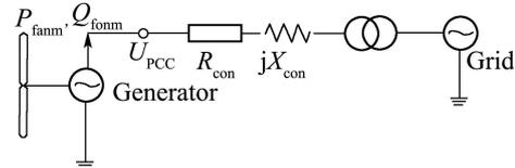
Fig. 7 Connection circuit between wind farm and stiff grid
