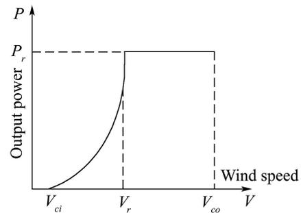
Fig. 4 Output power of wind turbine
