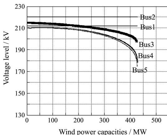
Fig. 14 Maximal wind power connected to weak grid
