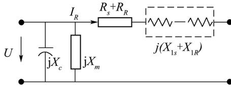
Fig. 5 Static model of wind turbine
