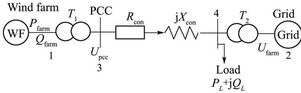
Fig. 10 Wind farm connected to “stiff grid”
