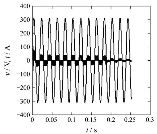
Fig. 12 The input voltage and current of matrix converter
