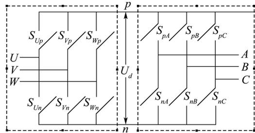
Fig. 2 The equivalent topology of 3-3 matrix converter
