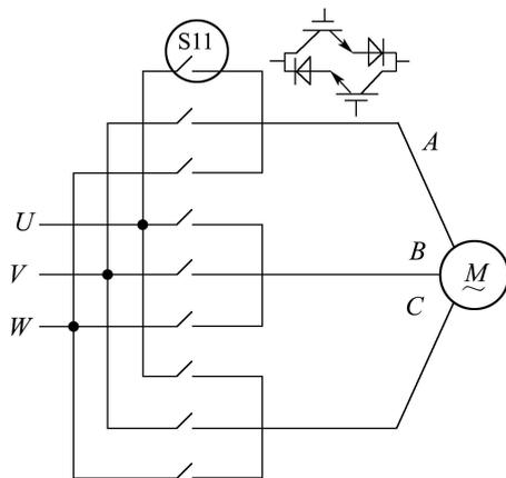
Fig. 1 The simplified topology of 3-3 MC
