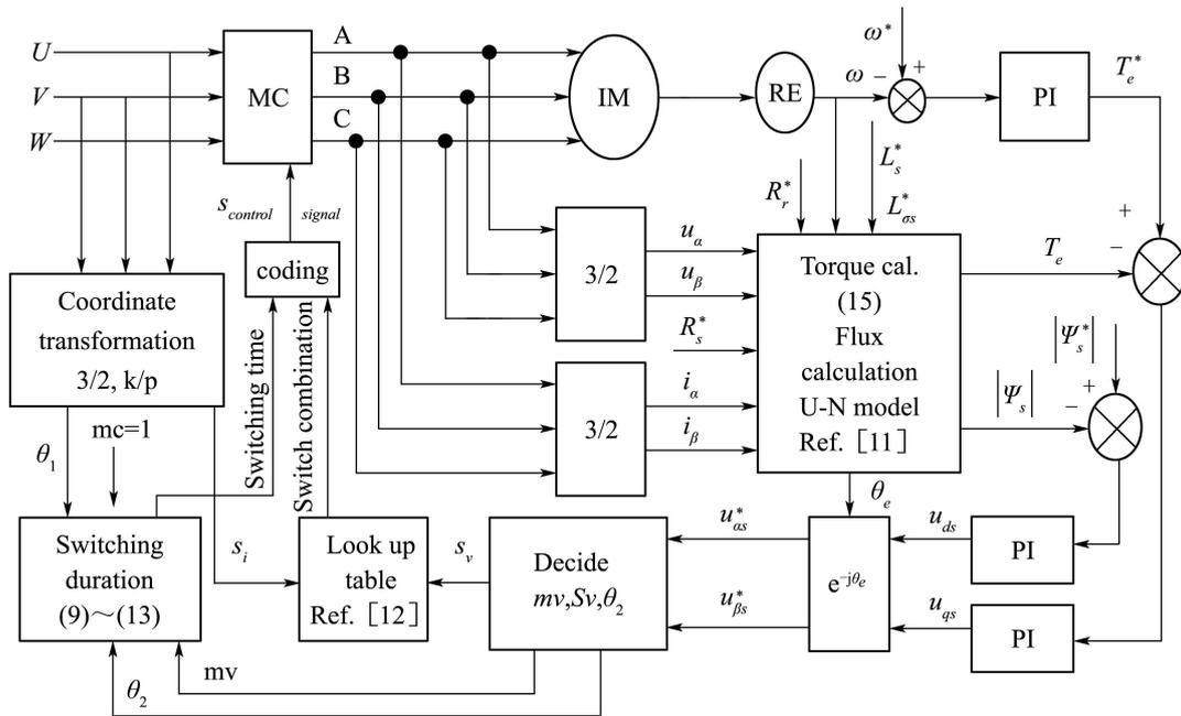
Fig. 4 Matrix converter-DTC novel control strategy system based on PI controller
