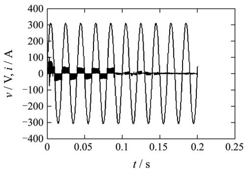
Fig. 6 The input voltage and current of matrix converter
