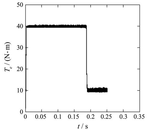
Fig. 11 The waveform of electric magnetic torque
