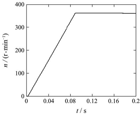
Fig. 7 The response of rotating speed of induction machine
