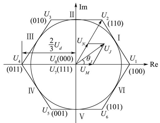
Fig. 3 The composition of output voltage vectors and its switching states
