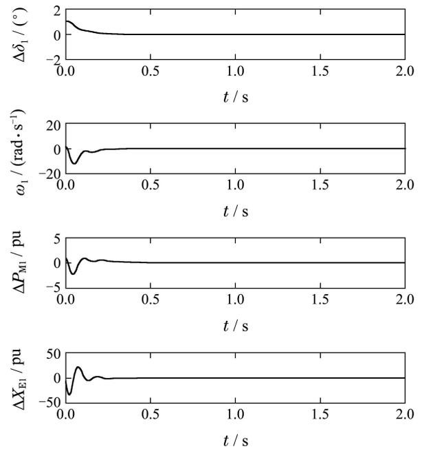
Fig. 6 The state trajectories for the generator #1 with the presented controller in Theorem 2
