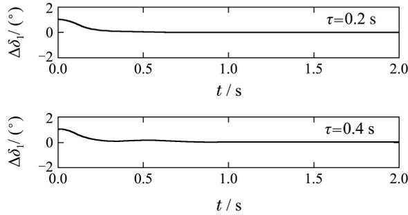
Fig. 5 The increment of rotor angle trajectories of generator #1 with various constant delays
