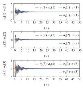
Fig. 2 The attitude error  $\sigma_i - \sigma_1 (i = 2, 3, 4)$
