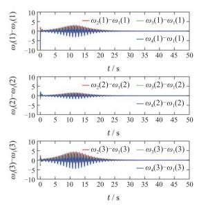
Fig. 3 The angular velocity error  $\omega_i - \omega_1 (i = 2, 3, 4)$
