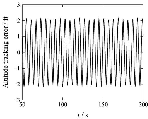
Fig. 4 Steady state tracking error of altitude
