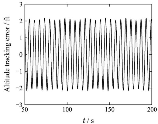
Fig. 8 Steady state tracking error of altitude
