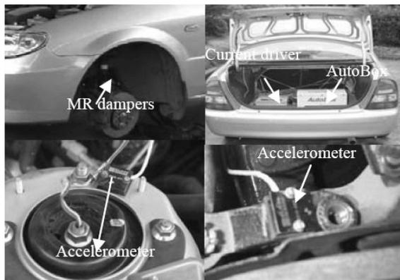
Fig. 6 Setup of the test car
