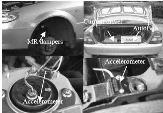
Fig. 6 Setup of the test car
