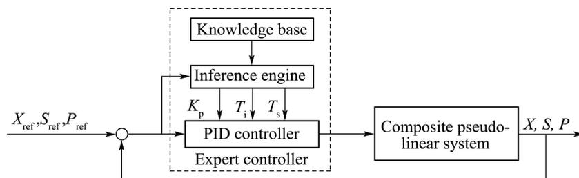
Fig. 2 Principle of expert controller
