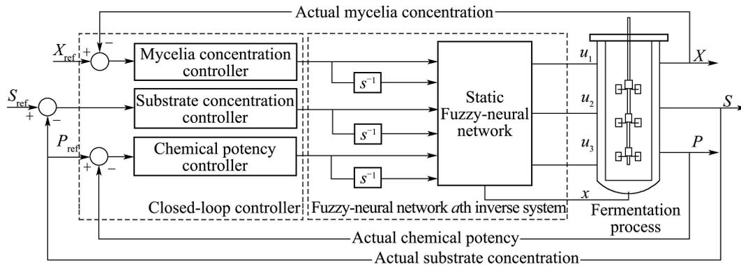
Fig. 3 Closed-loop structure of bioprocess using fuzzy-neural network  $\alpha$ th-order inverse decoupling control
