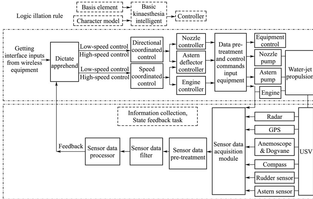
Fig. 2 Software architecture of the basic motion control system
