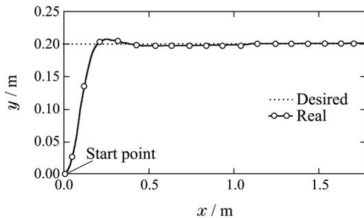
Fig. 5 Experimental result for the straight line tracking
