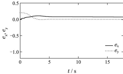
Fig. 6 Position errors for the straight line tracking
