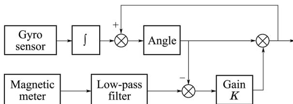
Fig. 3 Structure of estimate algorithm
