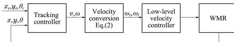
Fig. 1 Kinematics controller for the path tracking of WMR
