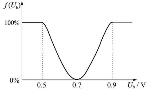
Fig. 4 Normal fault degree curve of  $U_b$
