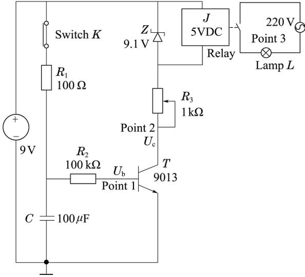
Fig. 3 Analog circuit
